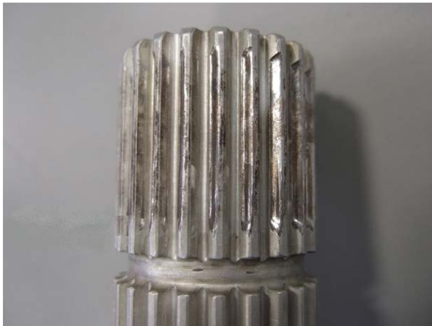
Example of the wear found on the tail rotor output wheel spline
