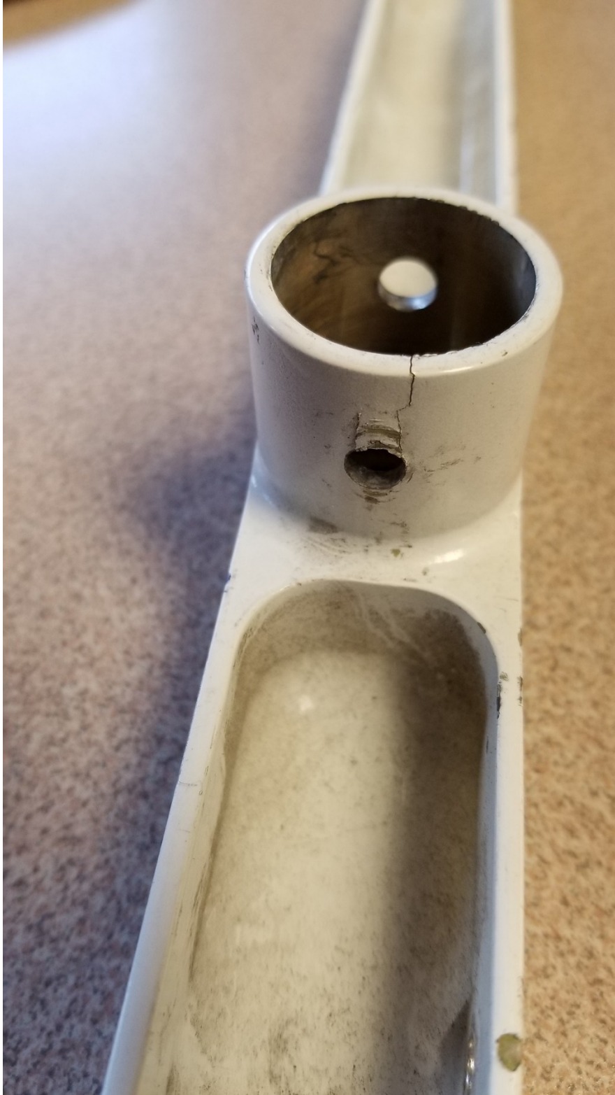
Fig. 3: Cracking and stress at pivot point
