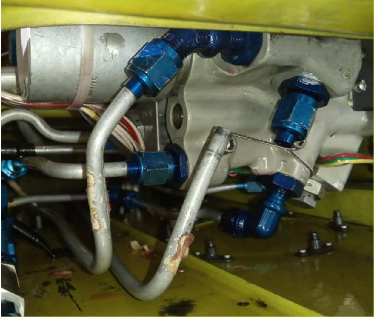
Hydraulic door open tube assembly failure at flare
