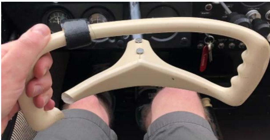
Cracked Plastic Control Wheel
