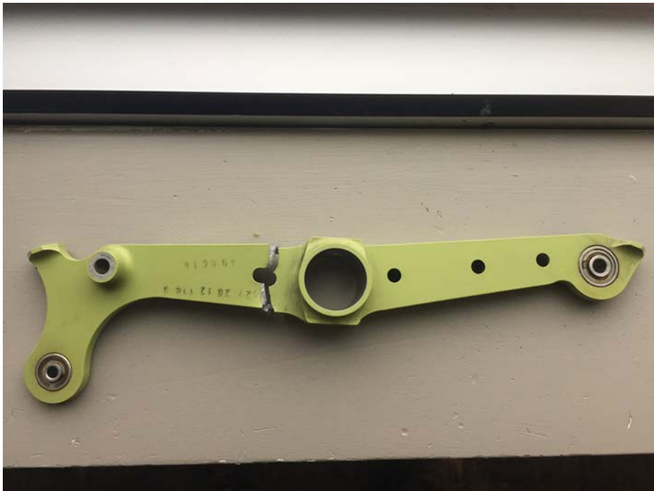
Pic. 2 Bellcrank removed on bench. Crack evident.
