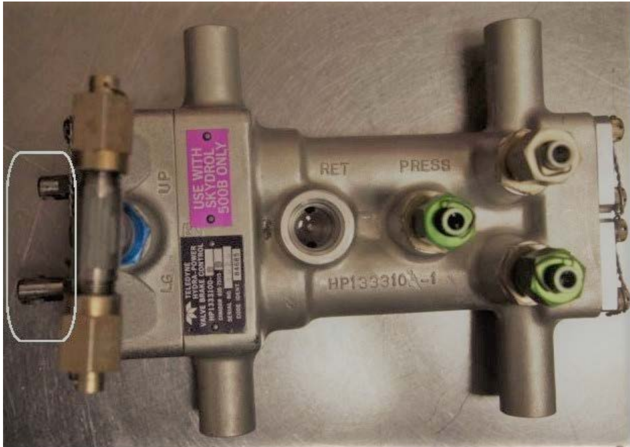
Fig 1: BCV showing misalignment of valve plunger positions.
