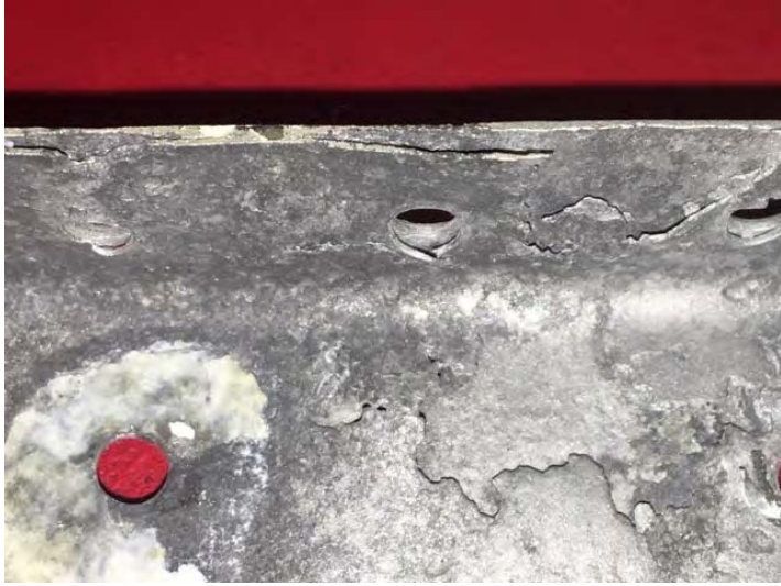
Fig 2: Close-up of corrosion showing depth and flaking
