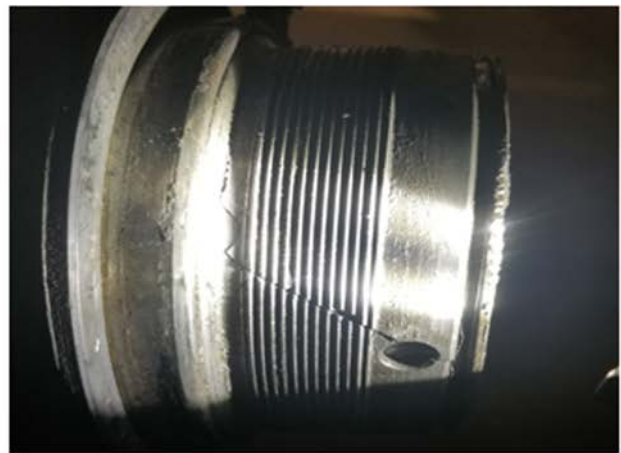
Close-up of main landing gear axle with axle nut removed
