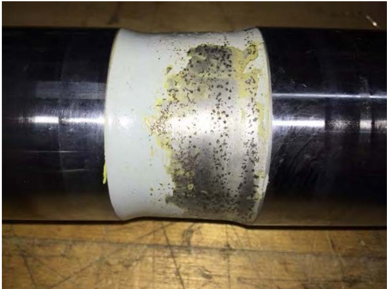
Pitting on the painted part of the axle
