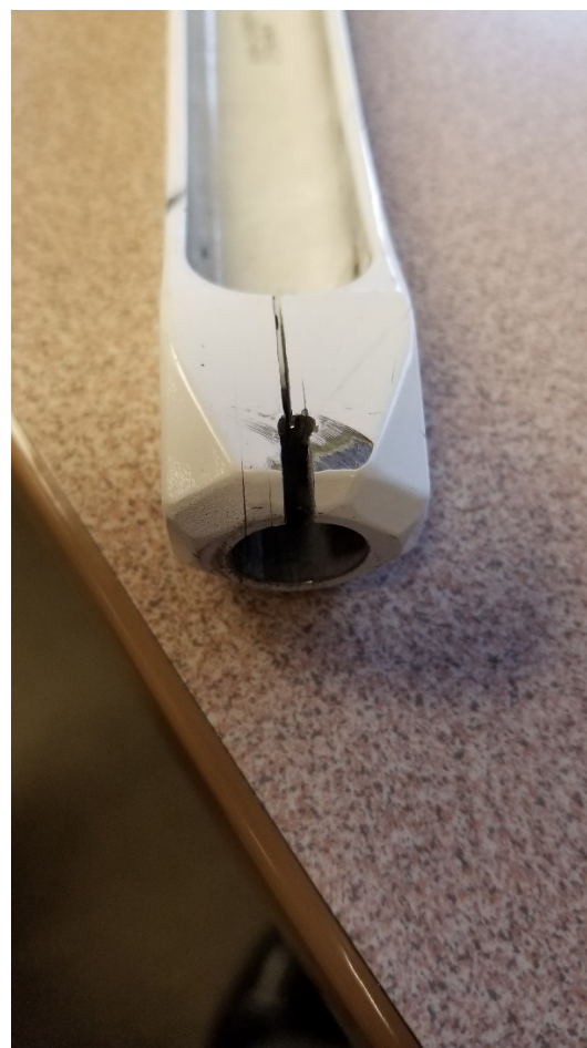
Fig. 2: Lever crack through taper pin hole
