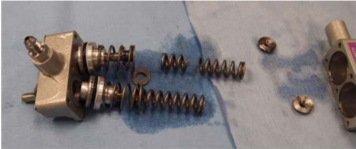
Fig 3: Close up of broken spring of the BCV.
